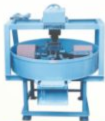
Muller Machine Cap. 50kg., 1 Ton
