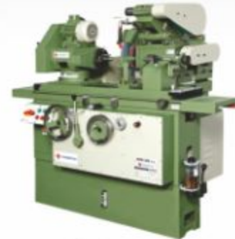
Cylindrical Grinding Machine 150 x 300 mm
