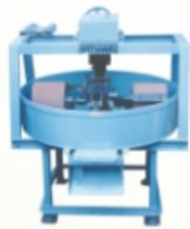
Muller Machine Cap. 50kg., 1 Ton
