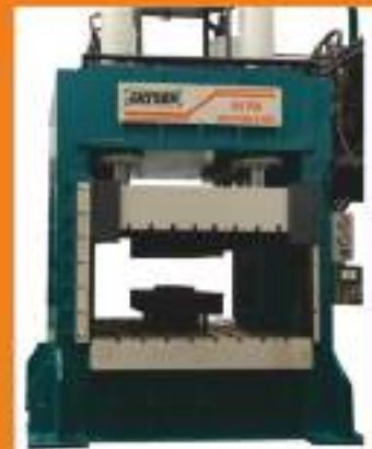
Deep Drawing Hydraulic Press ( 450 Ton )
